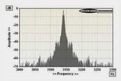
ABOVE: Wow and flutter re. 3150Hz tone at 5cm/sec (plotted  $\pm$ 150Hz, 5Hz per minor division). The -0.32% absolute pitch error will be inaudible
